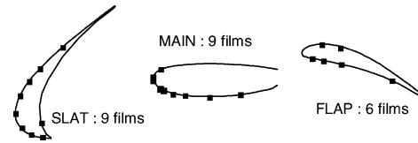
Fig. 2 Hot films locations on the AFV model (elements not to same scale).
